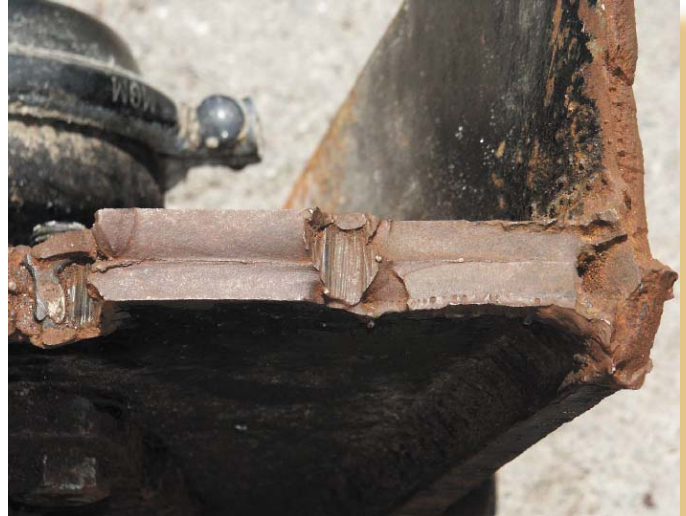
Reverse bending fatigue failure of an automotive component:
